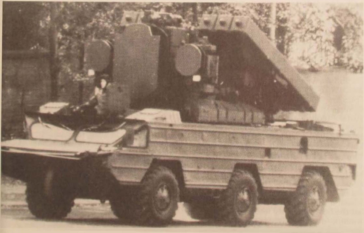
The SA-8—a short-range, low-altitude tactical surface-to-air missile—replaced the Soviets' 57-mm antiaircraft gun.
